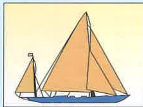
YAWL - Dua mast, mast belakang pendek lokasi di belakang rudder, rig jenis fore-and aft
